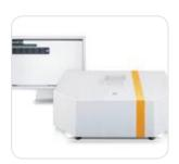
**SpeedCal Advantages at a Glance** Testing is carried out gravimetrically according to EN ISO 8655/6.
